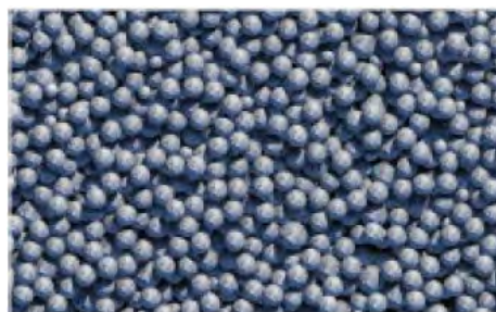
Figure 5. Conventional hydraulic fracturing methods rely on larger proppant sizes and resin coating to improve conductivity [9].
