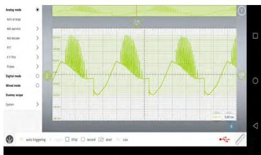
Figure 12. Triac controlled resistive load current waveform (Smart Scope).
