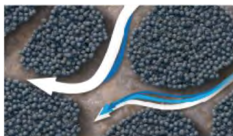
Figure 6. The HiWAY technique create stable, infinite-conductivity flow channels within fractures [9].
