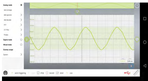
Figure 10. Resistive load (incandescent light bulb) current waveform (Smart Scope).
