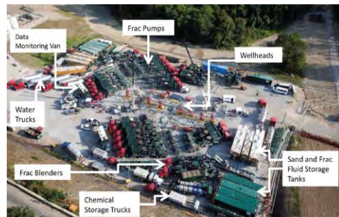
Figure 3. Huge numbers of tracks, equipment and large volume of fracturing fluid is need for staged hydraulic fracturing [5].
