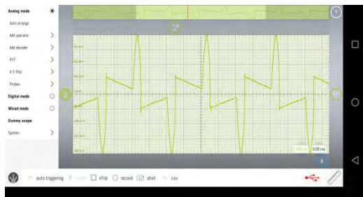
Figure 11. TV set current waveform (Smart Scope).
