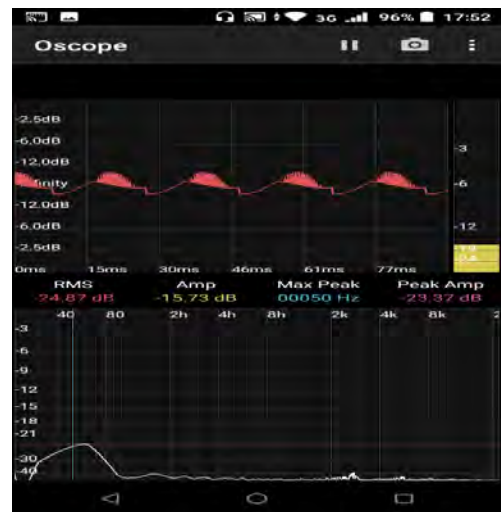
Figure 9. Resistive load high power - current waveform and frequency spectrum (Oscoscope).
