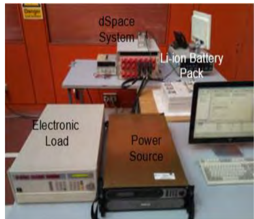
Figure 7. HIL test bench.
