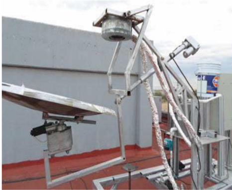
Figure 12. Solar tracker physically armed.
