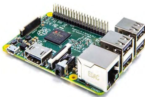
Figure 3. Raspberry Pi single-board computer
